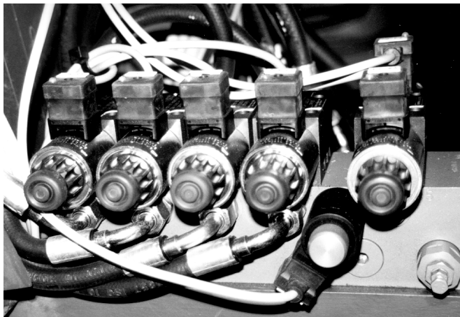
Figure 3: Control block all-wheel-steering
