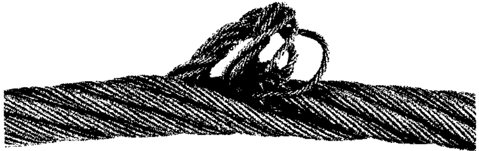
Figure 54. Improper handling, rope rotation or sudden release of a load can cause a 'popped core'.
