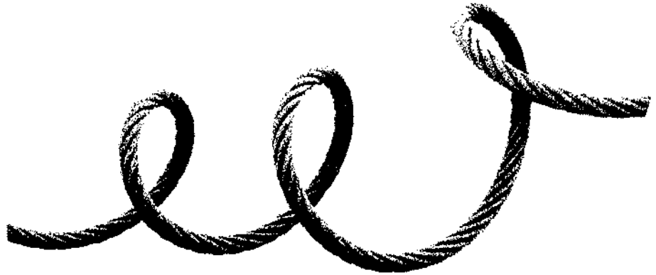
Figure 45A. A tightly spiralled “pig-tailed” rope; this condition is often the result of the rope being pulled around an object that has a small diameter.
