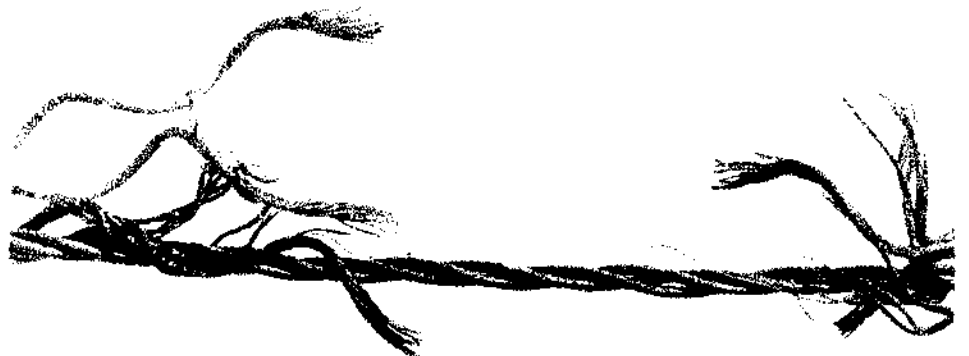
Figure 58. This is the appearance of a typical tension break on a test sample broken in a tensile machine. Note, not all strands have failed as the load relaxes when the initial few strands and/or the core fail.
