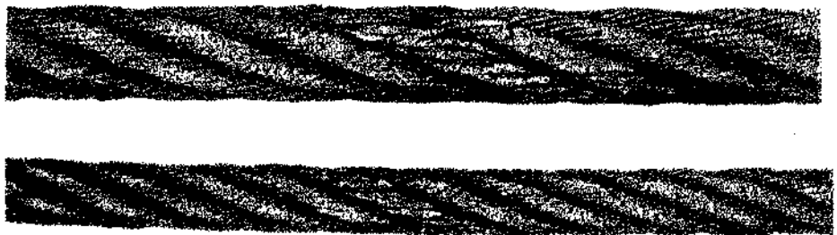
Figure 48. Wire rope with a high strand. In this condition, one or two strands are worn before adjoining strands. This is caused by improper socketing or seizing, kinks or doglegs. The top illustration (a) is a close view of the concentration of wear, the lower (b) shows how, in a six-strand rope, this recurs in every sixth strand.
