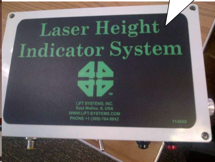
One gateway that that lasers connect too so the information can be sent to the display.
