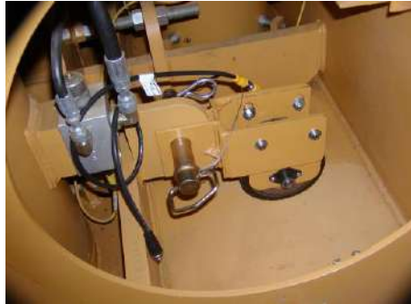
Figure 6.4 - Storage of Encoder Wheel
